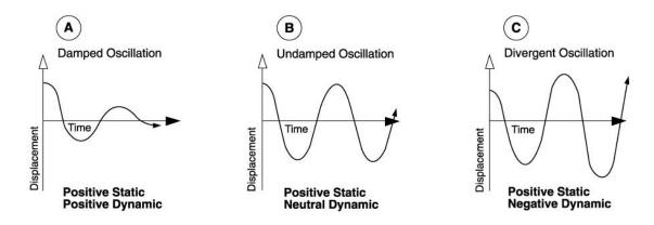
**Positive Stability:** The aircraft is able to return to its original attitude without any corrective measure.
