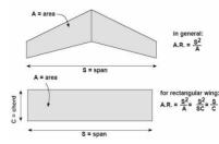
**Aspect ratio:** The relationship between the length of the wing and its width (chord). It is calculated by dividing the span by the average chord.
